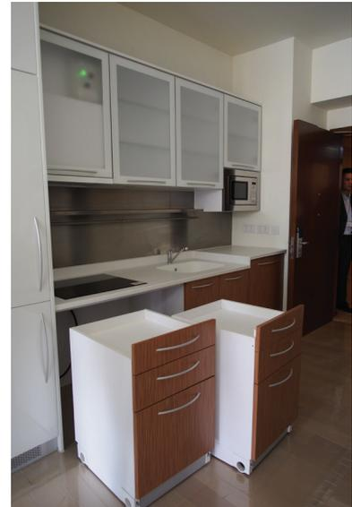
*[Fig. 7A.7] The design of this kitchenette has removable lower cabinet for adaptive use by people on wheelchair.*
