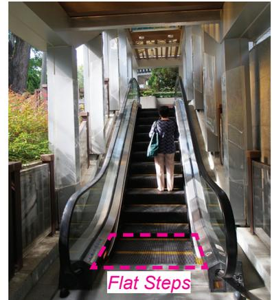
*[Fig. B7.1] Flat step is a step that is level with the landing prior to rising or descending along the incline.*
