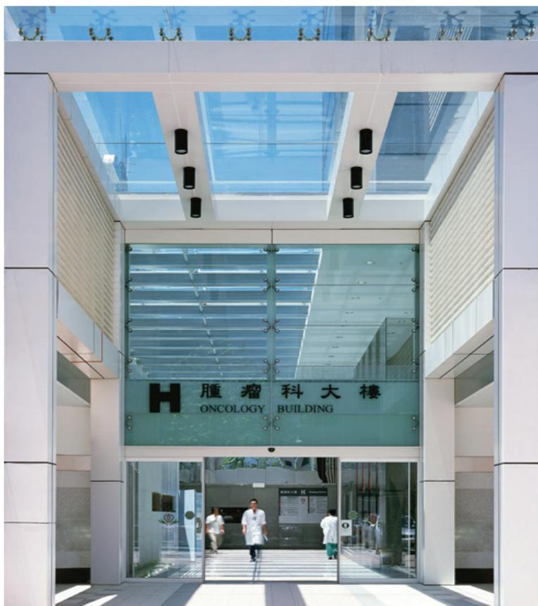
*[Fig. C3.2] Automatic door should be provided at main entrance of public building. Outside the entrance doors, adequate weather protected space should be provided to enable the visitors to get themselves ready before entering or after leaving the building. (Princess Margaret Hospital, HK)*
