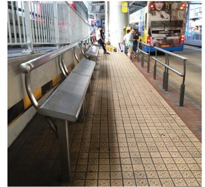
*[Fig.7D.1] Leaning bench is a space-saving design that is commonly used at busy bus station to provide a temporary resting point for riders.*
