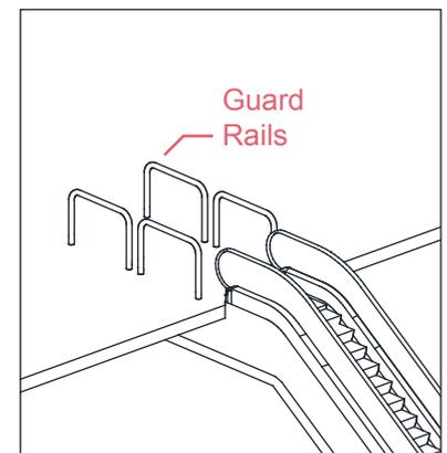
*[Fig.7D.2] Extended guide rails are recommended to create a safe transitional zone at landing area of escalator in crowded area.*
