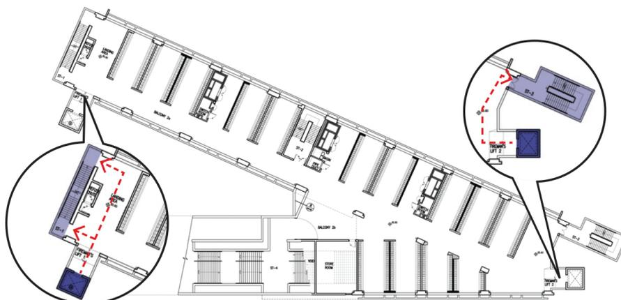
*[Fig. 7F.2] - Lift should be located adjacent to stairs for convenient use by the elderly. (Diamond Hill Columbarium, HK)*
