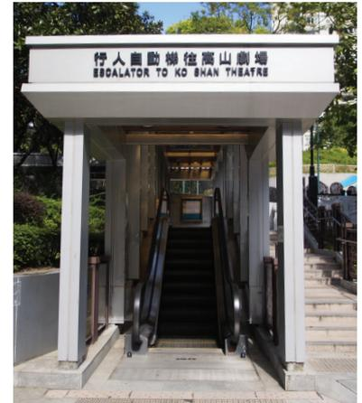
[Fig. B1.1] A weather protected escalator should be considered if there is substantial level difference between street and building levels.
