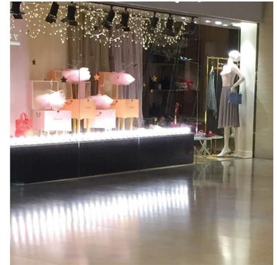
*[Fig. C1.1] Shiny and reflective floor finishes can be visually challenging for people with visual impairment. Shiny surface may give an impression of wet and slippery floor that is not safe to walk on. A dark patch may be mistaken as a hole or change in level.*
