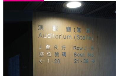
*[Fig. D1.4] Signage with reflective surface can cause glare and should be avoided.*
