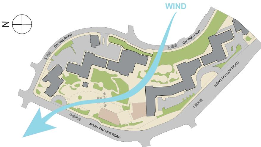
*[Fig. A4.1] The disposition of residential buildings takes consideration of the prevailing wind to enhance natural ventilation. (Upper Ngau Tau Kok Estate, HK)*
